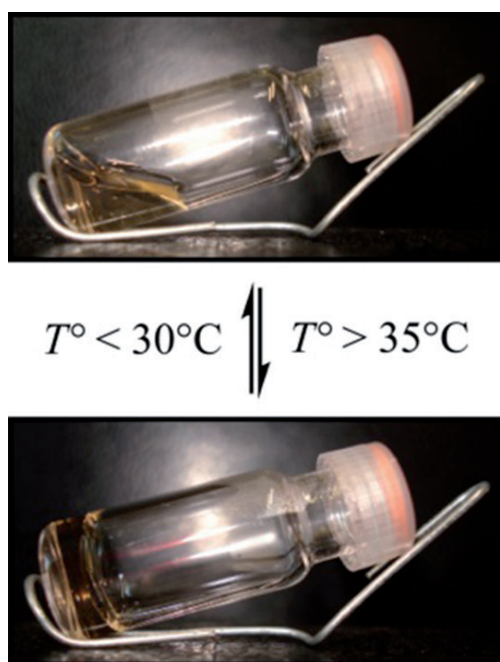
Figure 8: Pictures showing the thermo-induced assembly and disassembly of a coordination micellar gel
